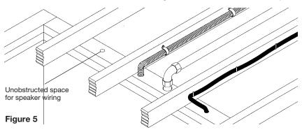
the drywall section can be replaced cleanly if there is an unseen obstruction behind the wall. BE VERY CAREFUL NOT TO SAW THROUGH EXISTING WIRES, PIPES, OR STRUCTURE. IF YOU FEEL ANY EXTRA RESISTANCE AS YOU ARE CUT-TING, STOP.
